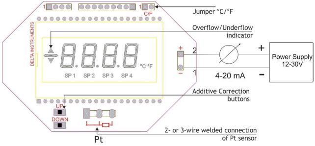
To connect the analog output and power supply, use pins 1 and 2 of the detachable cable plug, as shown on the diagram: 1 is – and 2 is +.
